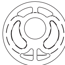
Proper elastomer sleeve orientation.
