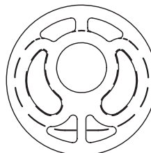
Proper elastomer sleeve orientation.
