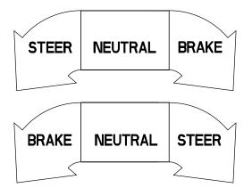
Pedal (F) – Brake and Steer functions (head end)
