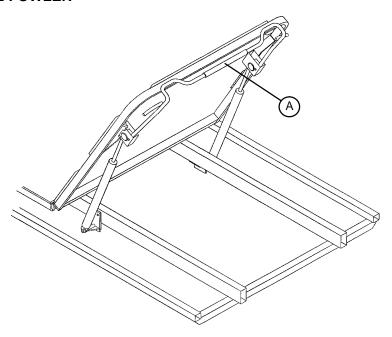
Squeeze handle (A) for pneumatic assistance in lifting the Fowler to the desired height. Remove hand(s) from handle when the desired height is achieved.
