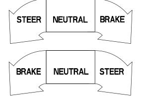
Pedal (D) – Brake and Steer functions (head end)
