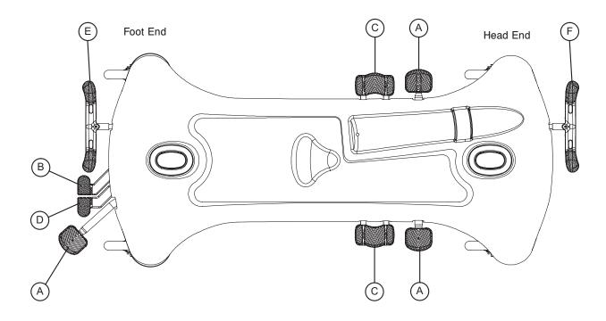
Pump pedal (A) at the foot end or sides of the stretcher to raise the litter
