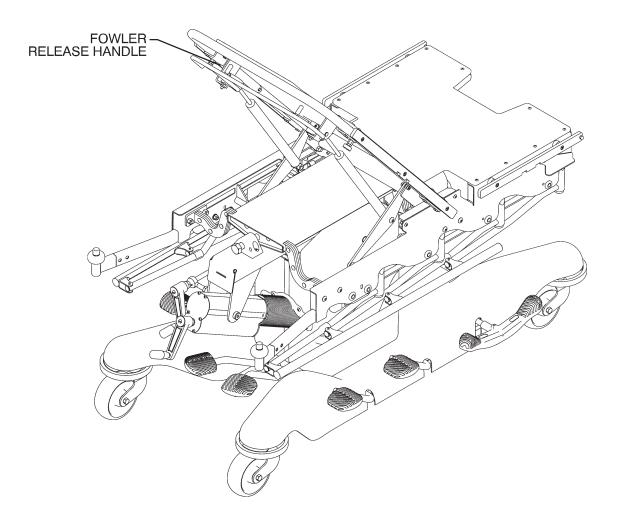
To Raise the Fowler: Squeeze the red handle under the Fowler for pneumatic assist in lifting the Fowler to the desired height. Remove your hand(s) from the handle when the desired height is achieved.
