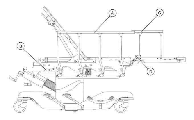
**To Engage the Litter Siderails**: Pull up on the top rail (A) of the litter siderail and raise it to the full up position until the latch engages with an audible click.
