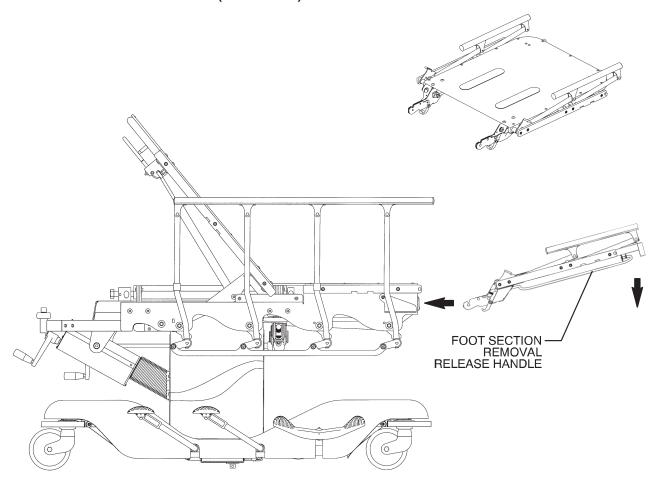
**To Remove the Foot Section**: For pelvic and lower body procedures, squeeze the red handles under the foot section on both sides and lift the foot section from the two receptacles at the end of the seat.
