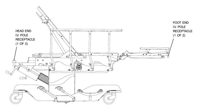
Two I.V. pole receptacles for use with standard I.V. poles are located at the head end of the unit on the Fowler and at the foot end on the foot section.
