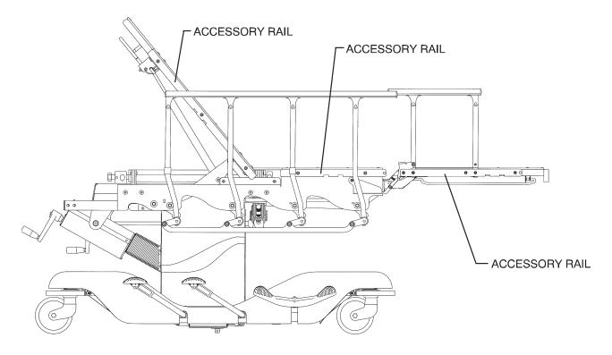
Accessory rails border the litter frame. Direct clamps and other ancillary surgery equipment may be attached to the rails.
