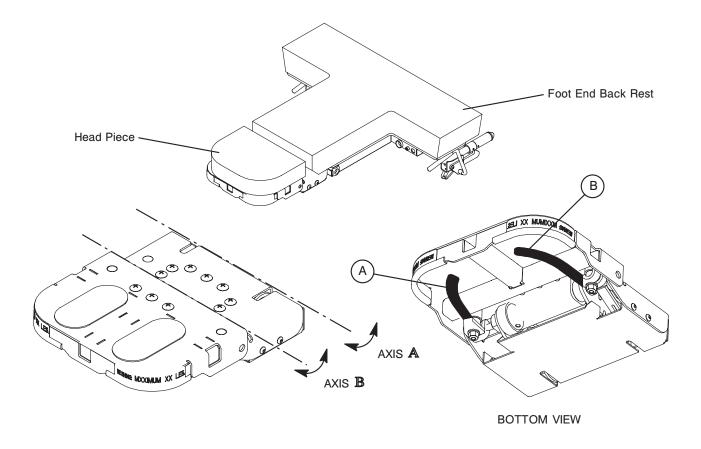
**To Operate the Articulating Head Piece**: Grasp either handle under the head section and squeeze. Handle (A) releases one latch and rotates the head piece on axis "A". Handle (B) releases the other latch and rotates the head section on axis "B". For ease of operation, it is recommended to release only one latch at a time.
