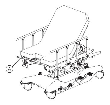
Tilt the cysto pan holder bracket (A) and insert it between the top and bottom roller bearings on the litter brackets.
