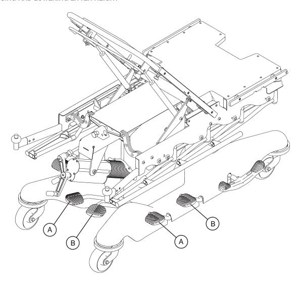
To Raise the Litter Height: Depress and release the litter up pedal (A) repeatedly until the desired height is reached.
