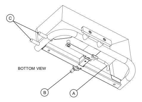
The Pre—Op/Post—Op Head Extensions are designed to be used only with the articulating head piece on the optional Foot End Back Rest to provide additional litter surface and to protect the patient's head during transport. The head extensions can be used as push handles when the Trio is being moved.
