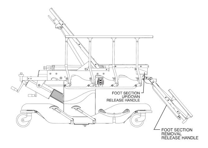
**To Lower the Foot Section**: With one hand, squeeze the foot section up/down release handle at the side of the foot end of the litter. With the other hand, push down on the foot section to move it to the desired angle.
