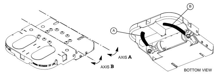
To operate the articulating head piece, grasp either handle under the head section and squeeze. Handle (A) releases one latch and rotates the head piece on axis "A". Handle (B) releases the other latch and rotates the head section on axis "B". For ease of operation, it is recommended to release only one latch at a time.
