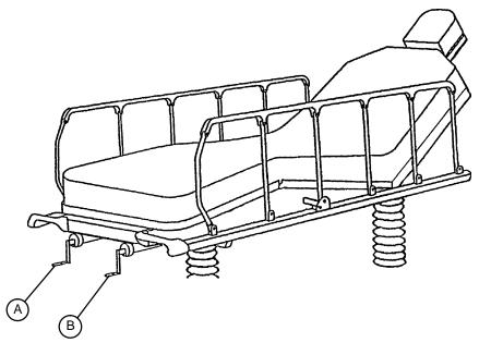
The Fowler and Gatch crank handles are stored under the litter and held out of the way with magnets. Pivot the crank out and push in to engage it.
