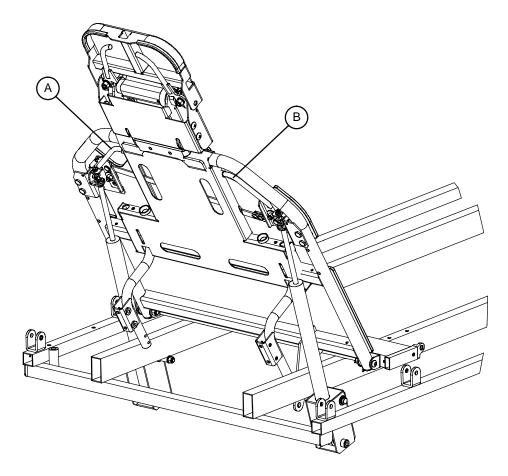
• Squeeze handles (A & B) for pneumatic assistance in lifting the Fowler to the desired height. Remove hand(s) from the handles when the desired height is achieved.
