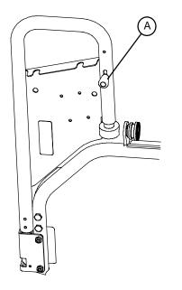
The Pre–Op/Post–Op Head Extensions are designed to provide additional litter surface and to protect the patient's head during transport. The head extensions can be used as push handles when the stretcher is being moved.
