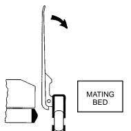
3. When the transfer board is fully raised, it can be pivoted downward onto the surface of the mating bed or stretcher.
