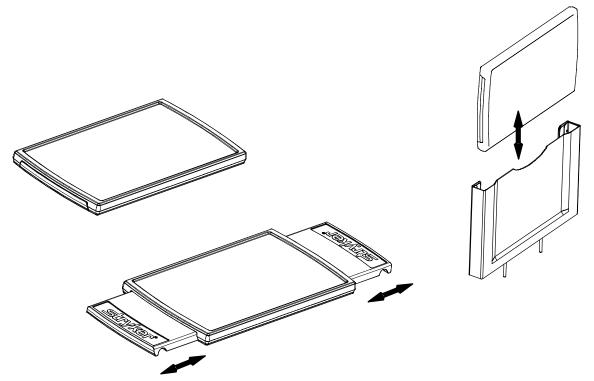
Pull out on either end of the serving tray to extend it to the proper width to fit on top of the stretcher siderails.
