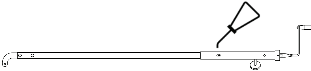
Figure 16 – Crank screw lubrication
