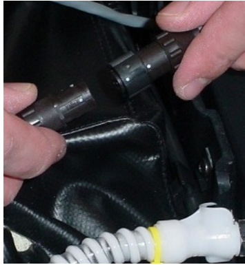
Figure 4: Connect the tilt sensor cables
