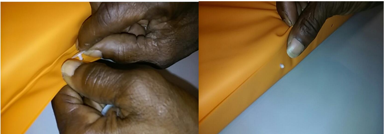
Figure 124: Insert Male Snap Rivet
