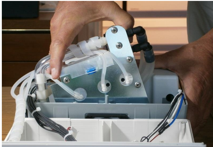
Figure 26: Valve Manifold Release
