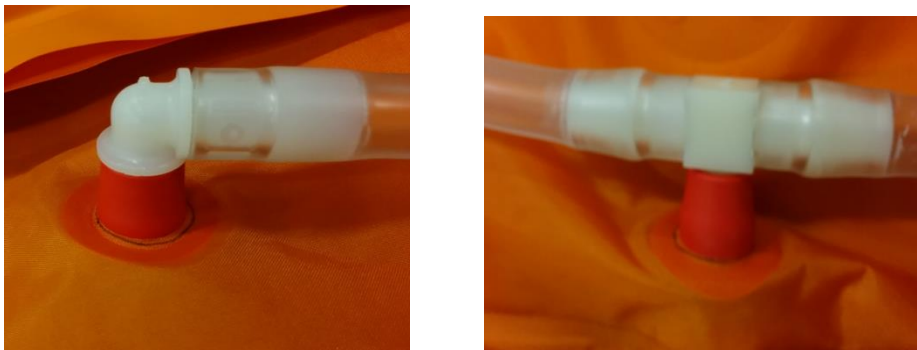
Figure 127: Fitting Inserted Into Flange
