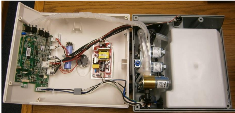
Figure 12: Pump Opened Laying Flat on Surface
