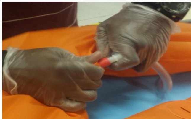
Figure 92: Removing Bolster Hose from Flange
