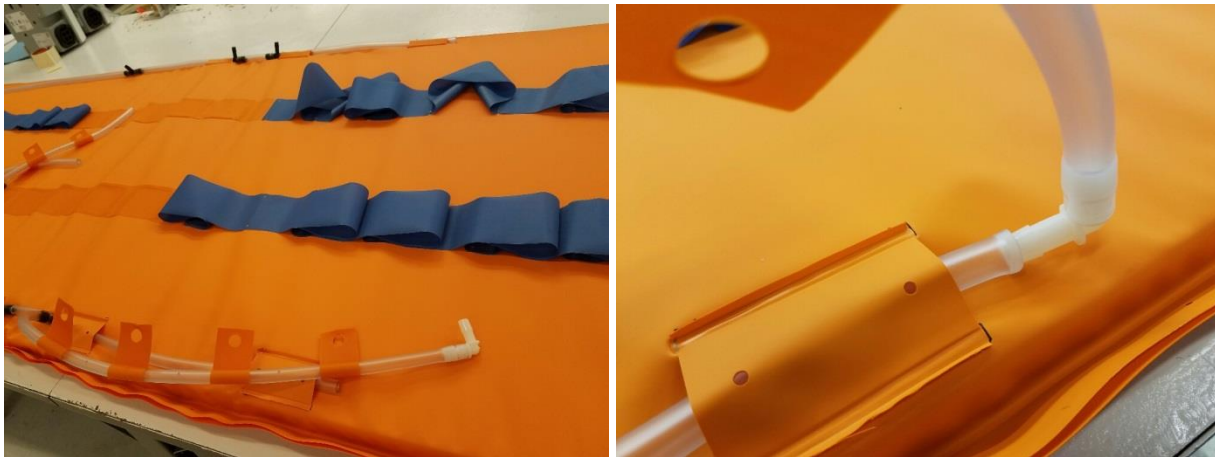
Figure 85: MM Hose Assembly
