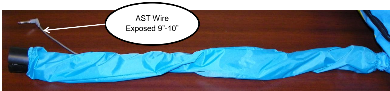
Figure 62: Exposed AST Wire
