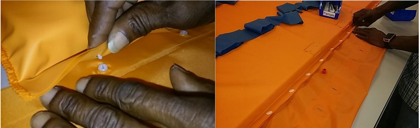
Figure 126: Attaching Bolster to Overlay
