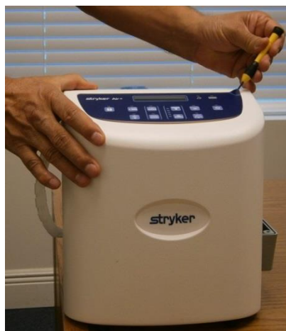
Figure 19: Touch Panel Removal
