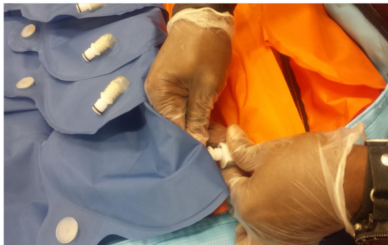
Figure 64: Disconnected Air Cells
