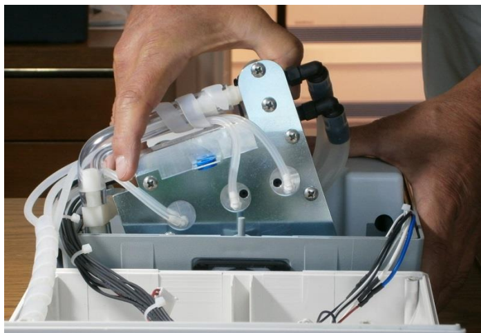
Figure 15: Valve Manifold Displacement
