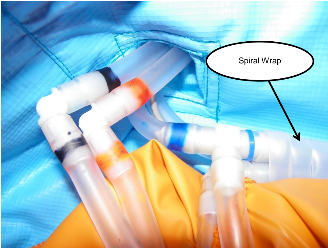
Figure 113: Hose Spiral Wrap (Located at Patient Right Foot Side of Mattress)
