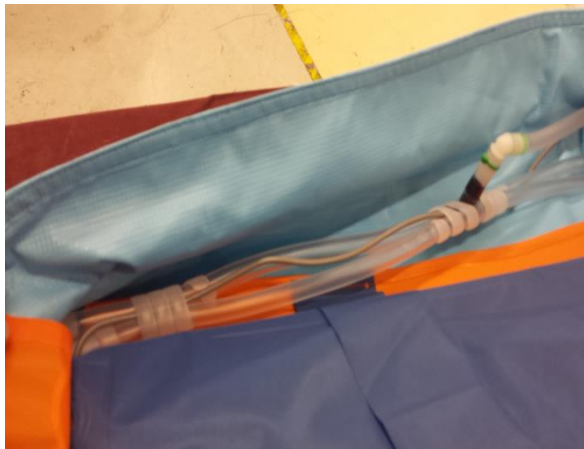
Figure 130: Bundle Hoses and Spiral Wrap
