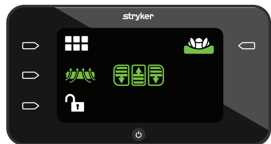
Figure 20 – Home screen, operator view
