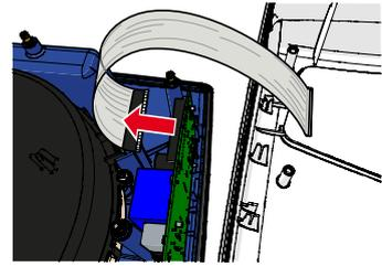
**9.** Secure the connector by applying hot-melt to the full width of the connector.
