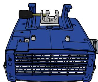
3. Remove the two screws of the filter cap with a 4 mm hex key.
