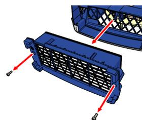
4. Remove the 9 screws which connect the front and back housing using a 3 mm hex key.
