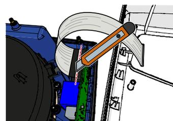
**8.** Remove the connector from the PCBA and attach the connector of the new front cover.
