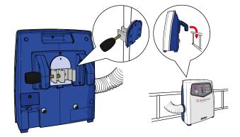
Quick-release mechanism to switch between mounting to bed rail/end and pole.
