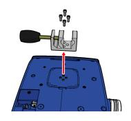
**7.** Optional: Mount the Wall mount and Cover plate to a wall using wall screws and plugs specifically designed for the used wall material (not supplied). First check the adequacy (of the surface) of the structure to which the wall mount will be attached based on the mass of the device (see *Specifications of the device* on page 39) and the center of gravity shown below.
