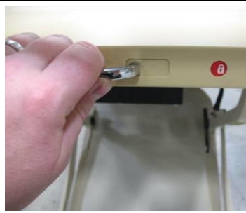
Knob not fully clamped (knob fastener not fully engaged)
