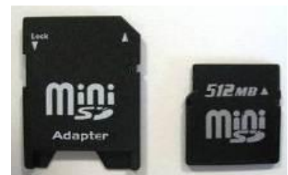
Example of miniSD card and SD card adapter used for CB10 firmware updates
