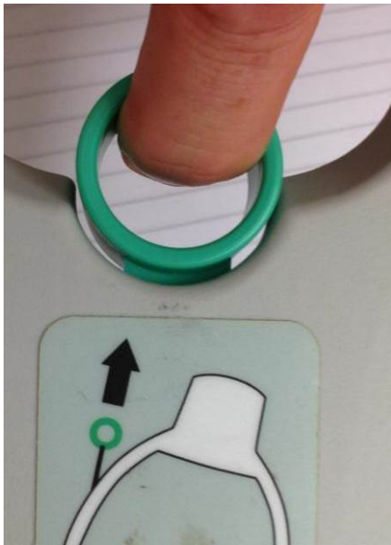
Figure 10.2-1: Release Ring Check
