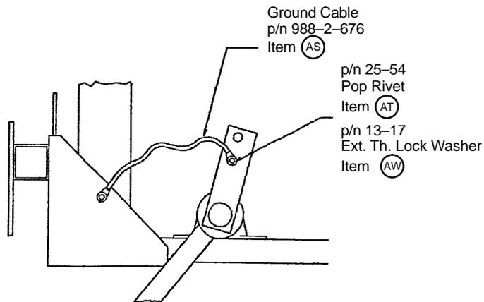
Side View of Pump Lever Arm and Base Tube Gusset Grounding Scheme
