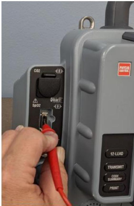
Connection **(F)** in the setup diagrams can be made by attaching a meter probe to the Safety Analyzer and holding the probe tip on the pin identified (pin 13) above during testing – as shown in photo at the left
