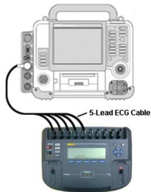
Figure 1.35—ECG 5-wire connection
