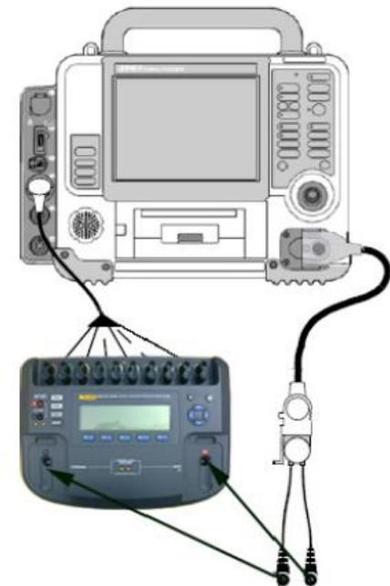
Figure 1.53—Pacer leads-off test setup
