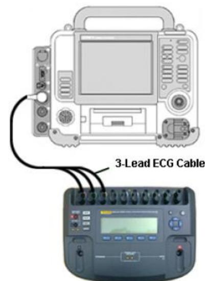
Figure 1.37—ECG 3-wire connection
