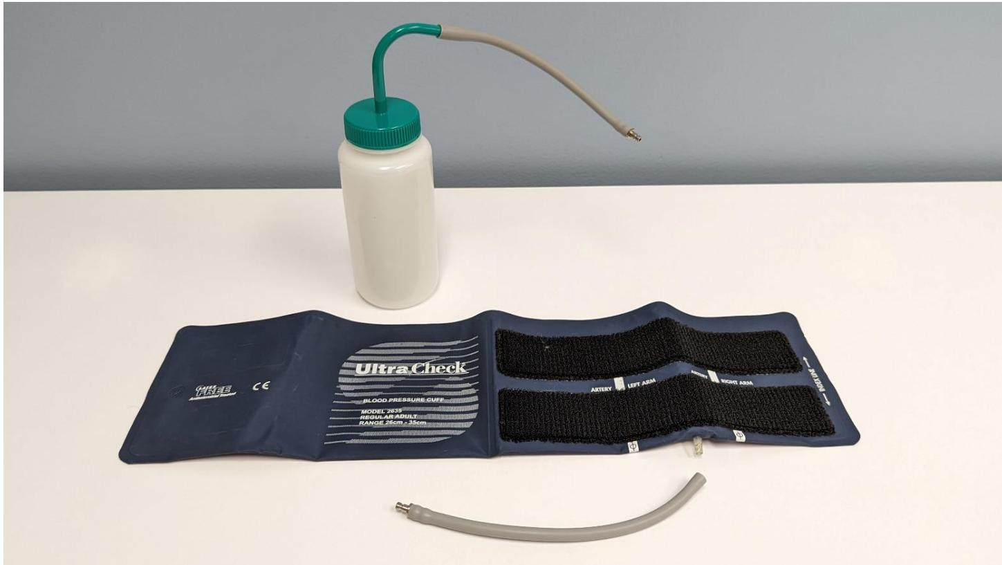
5. Install the removed hose onto the spout of the NIBP test bottle. It is recommended to rub a lubricant like dish soap on the bottle spout. This will allow the hose and spout to create a greater connection.
