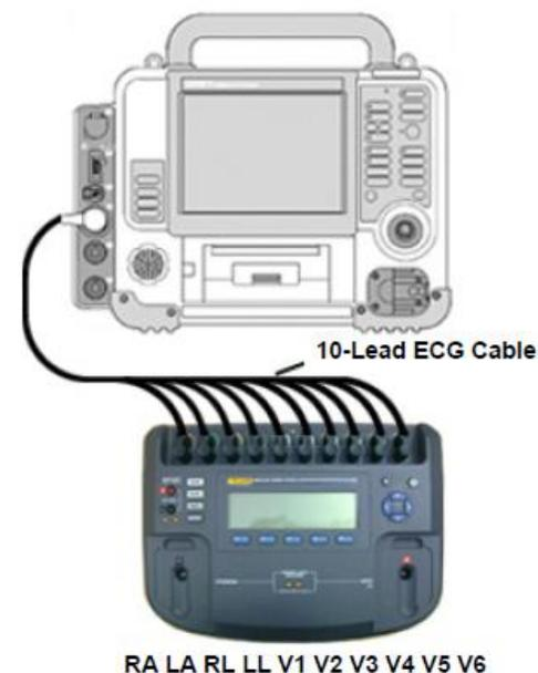
Figure 1.33—ECG lead connections
