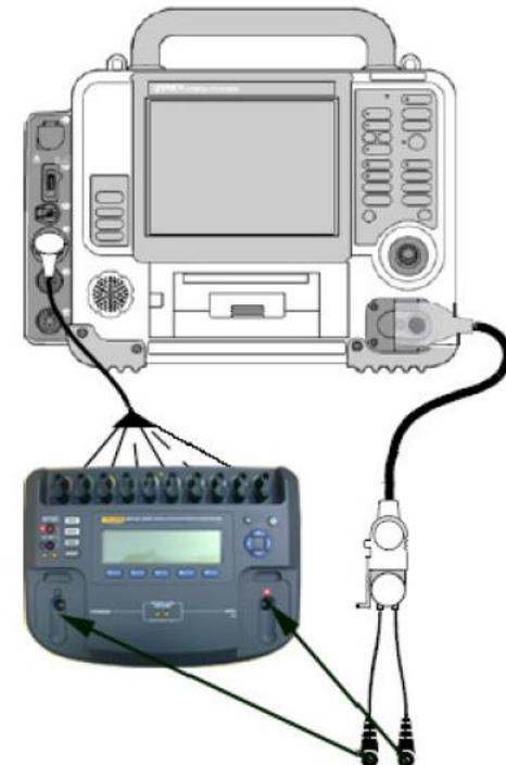
Figure 1.54—Pacer output current test setup
