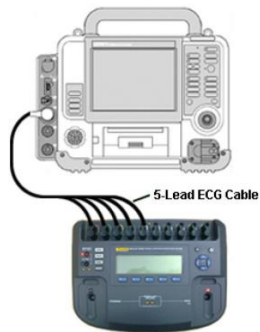
Figure 1.35—ECG 5-wire connection
