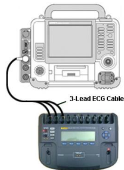
Figure 1.37—ECG 3-wire connection
