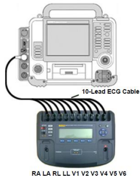
Figure 1.33—ECG lead connections
