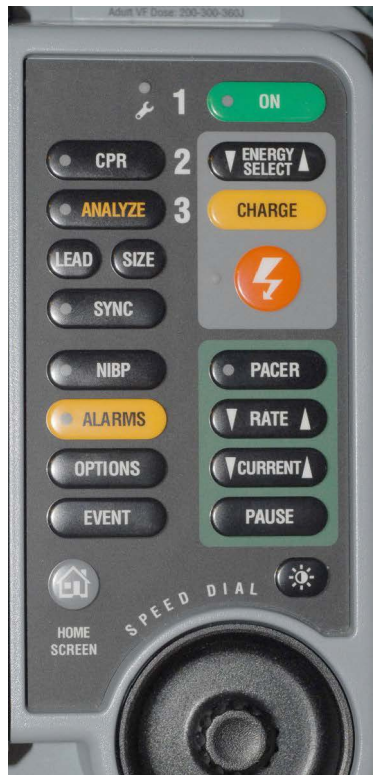
Figure 8.16—Main keypad replacement
