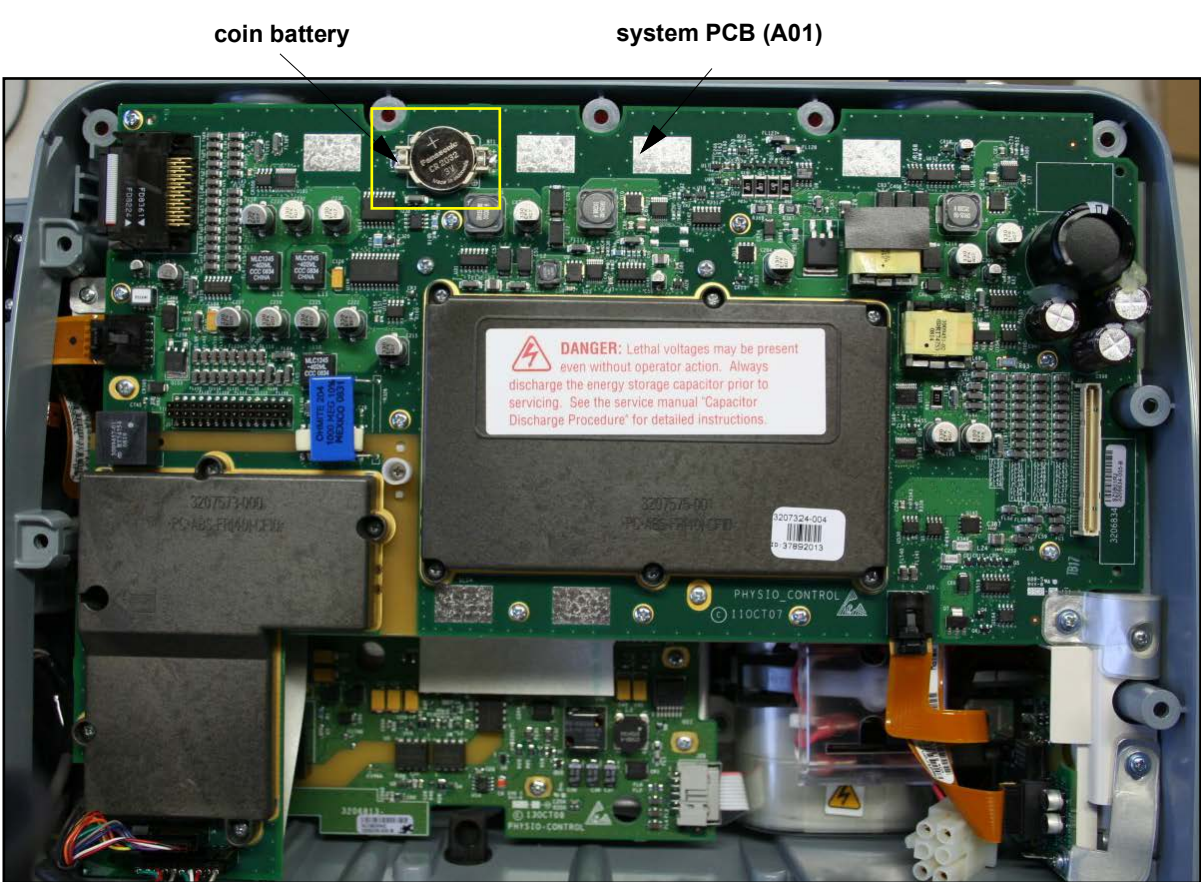
Figure 8.123—Coin battery location
