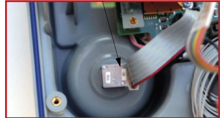
Figure 8.28—Speed dial assembly
