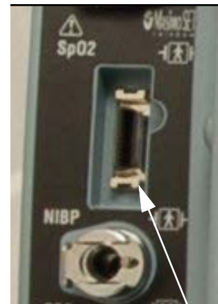
SpO2 connector orientation
