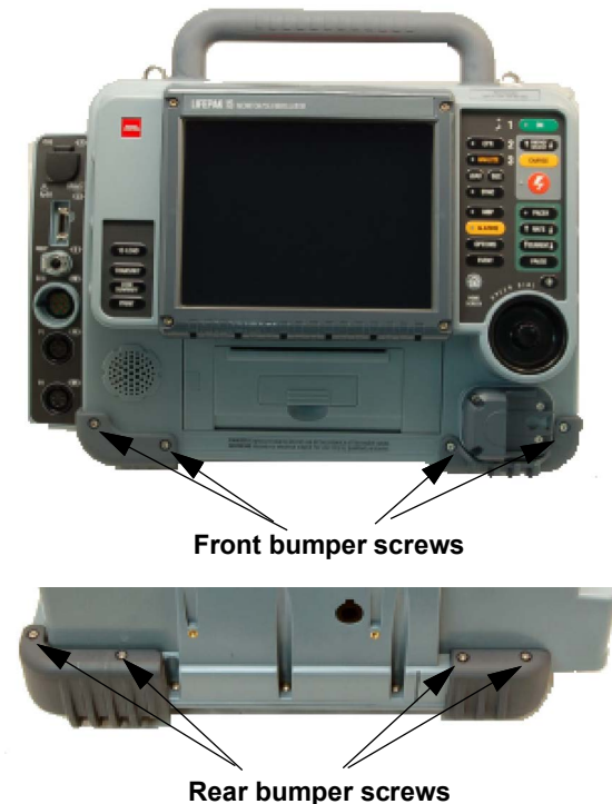
Figure 8.4—Bumper screw locations
