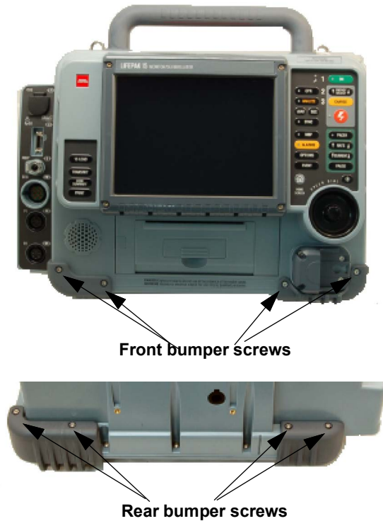
Figure 8.9—Bumper screw locations
