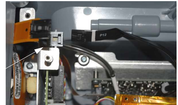
Figure 8.75—Power PCB J12 connection
