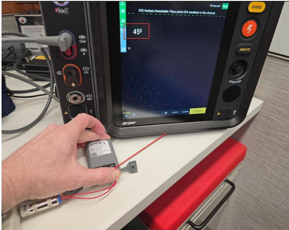
If the reading is still out of range, try testing on a different device or using a different temp cable. If it is determined that the device is the issue you can try replacing the temp connector or the system PCB.
