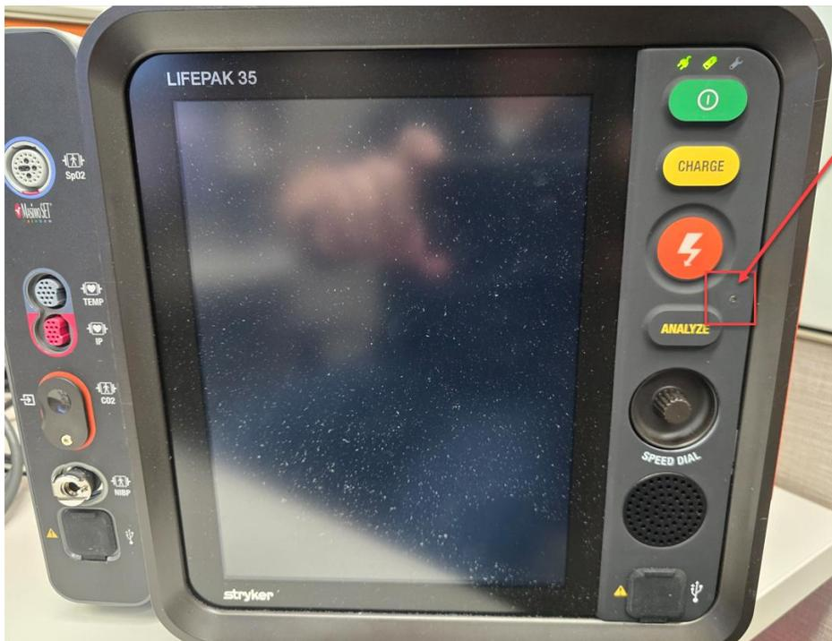
If you are working in an environment that has poor lighting it might help to shine a flashlight at the sensor at the beginning of the Ambient Light Sensor test to allow the application to register an adequate baseline reading.
