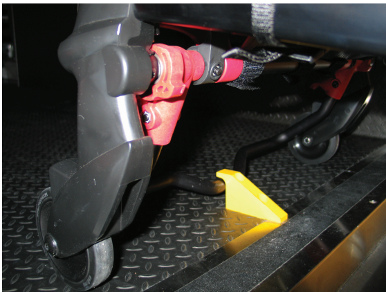
Figure 7 – Safety bar secured in the vehicle safety hook
