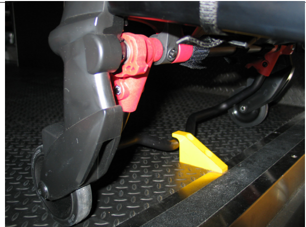
Figure 18 - Safety Bar Engaging the Safety Hook
