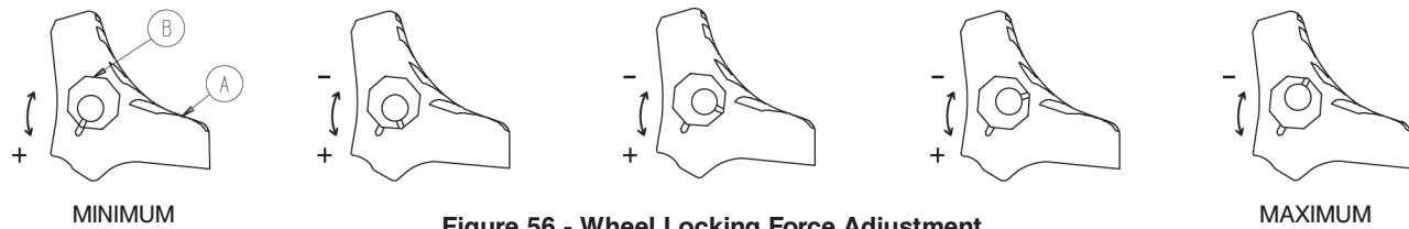
Figure 56 - Wheel Locking Force Adjustment
