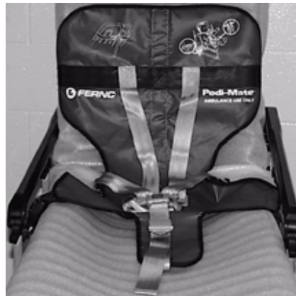
Figure 24- Pedi-Mate™ Strapped to a RUGGED Cot
