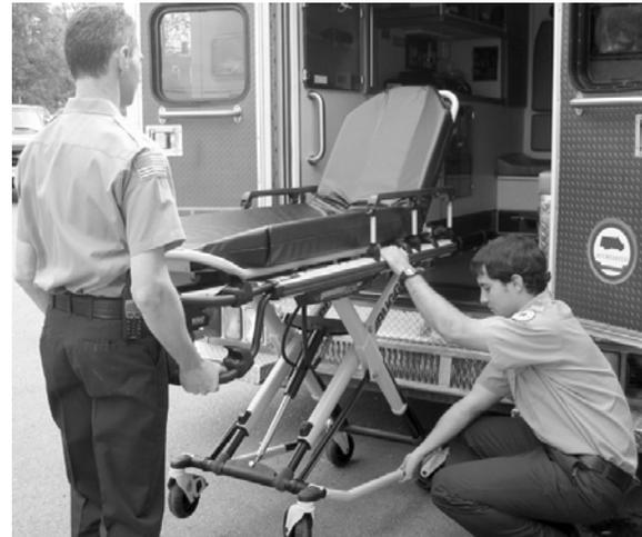
Figure 53 - 2 Operators - One Lifting the Base
