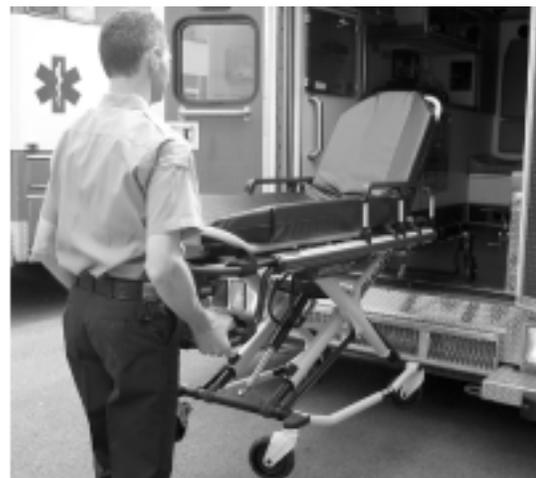
Figure 50 - Remove Load Wheels from the Vehicle Floor
