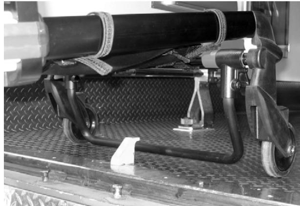
Figure 39 - Safety Bar Engaging Safety Hook
