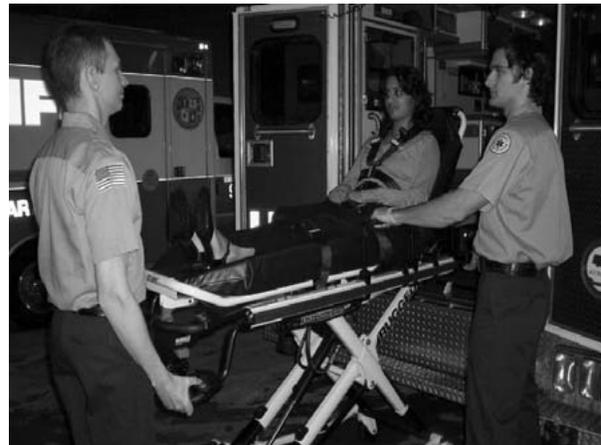
Figure 40 - 2 Operators - One Pushing the Retract Button
