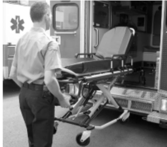
Figure 42 - Load Wheels on the Vehicle Floor
