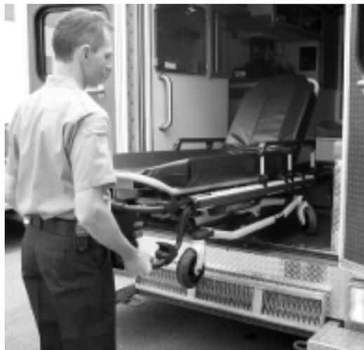
Figure 48 - Pull the Cot out of the Vehicle
