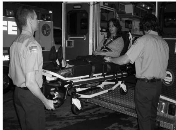
Figure 41 - 2 Operators Loading the Cot
