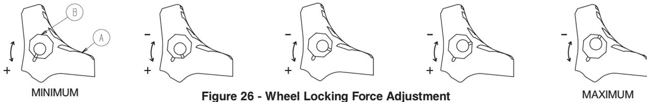
1. To adjust the wheel locking force, remove the socket screw from the center of the lock pedal. The wheel lock is initially assembled with the pedal set at the minimum locking force. The marker on the pedal (item A) is aligned with the marker on the octagonal sleeve (item B).
