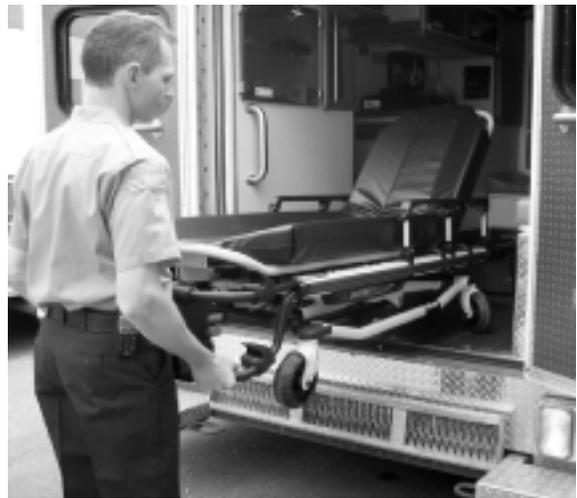
Figure 58 - Pull the Cot out of the Vehicle
