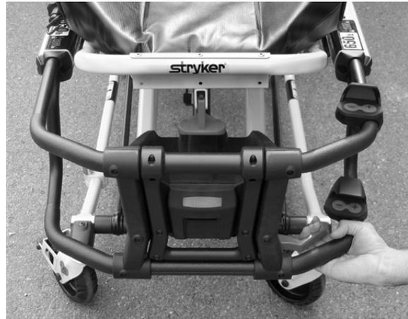
Figure 52 - Manual Release Lever
