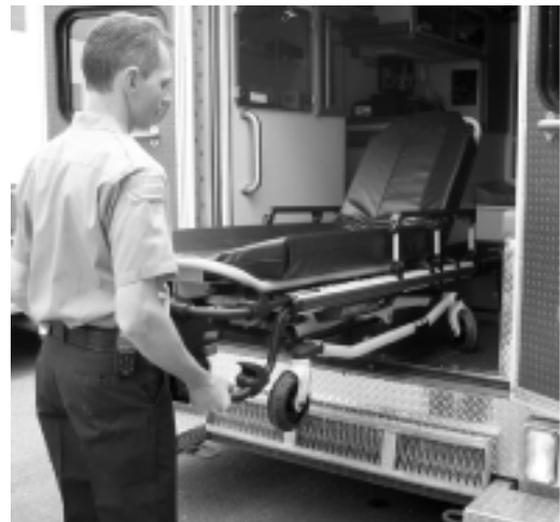
Figure 44 - Push the Cot into the Vehicle
