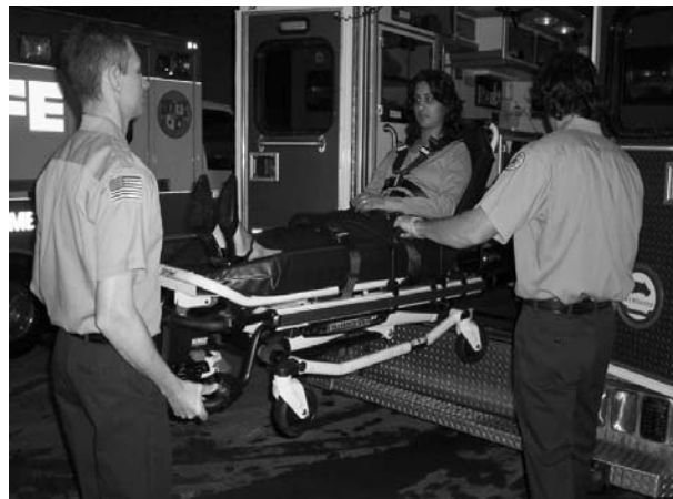
Figure 16: 2 Operators Loading the Cot
