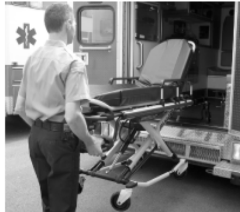
Figure 17: Load Wheels on the Vehicle Floor
