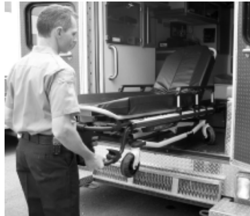
Figure 33: Pull the Cot out of the Vehicle
