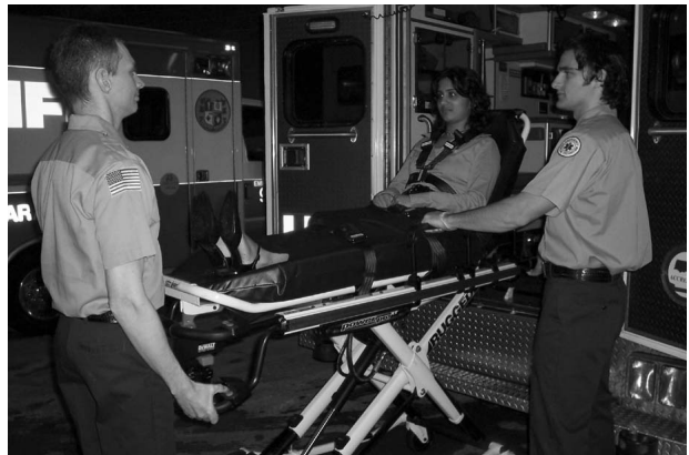
Figure 21: 2 Operators - One Pressing the Extend Button
