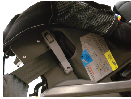
Figure 35 – Rear facing lock-off
