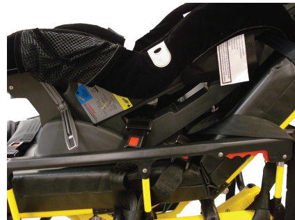
Figure 31 – Secure the waist restraint
