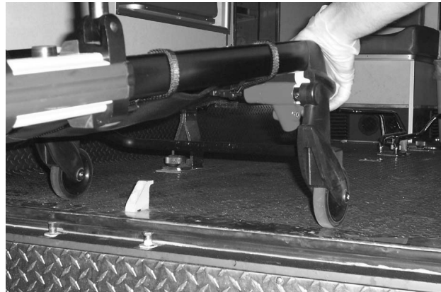
Figure 24 - Disengaging the Safety Bar
