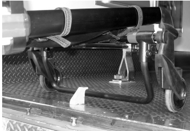
Figure 22 - Safety Bar Engaging Safety Hook
