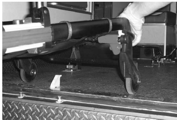
Figure 27 - Disengaging the Safety Bar
