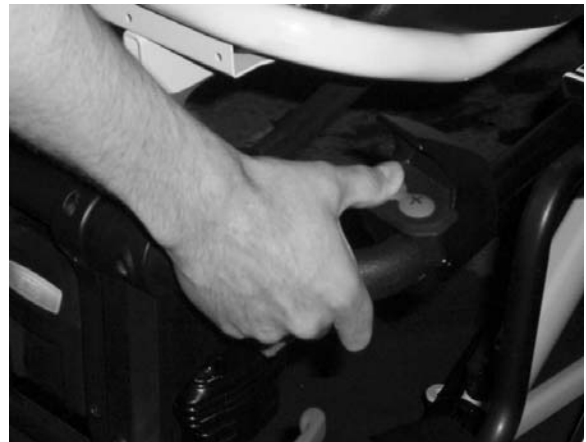
Figure 23 - Push the Retract Button
