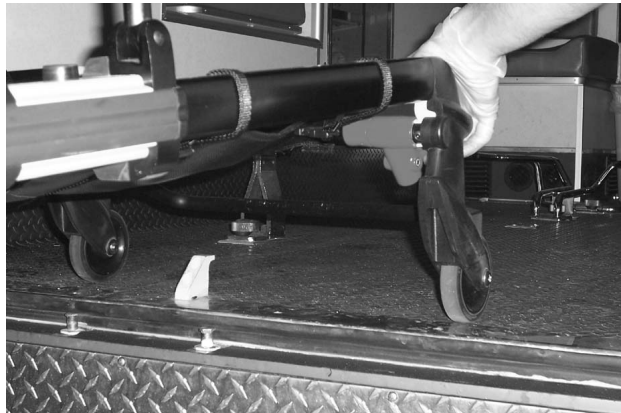
Figure 24 - Disengaging the Safety Bar
