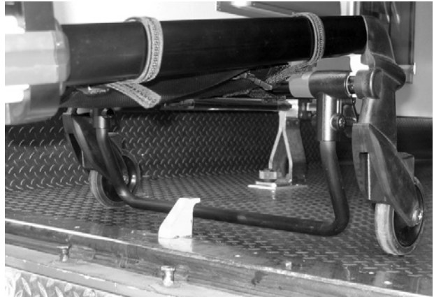
Figure 14: Safety Bar Engaging Safety Hook
