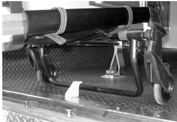
Figure 20: Safety Bar Engaging Safety Hook
