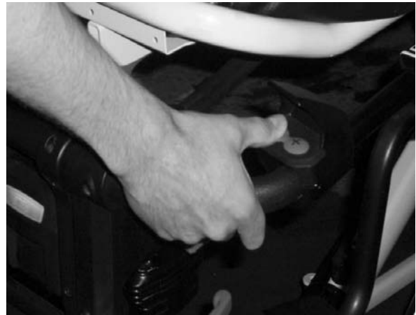
Figure 21: Press the Retract Button
