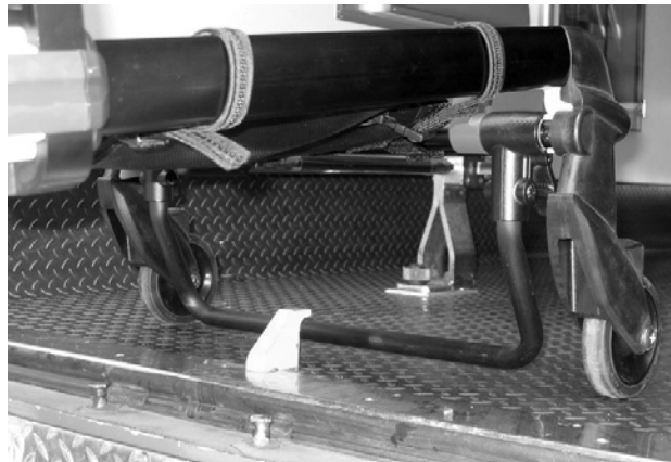
Figure 20: Safety Bar Engaging Safety Hook
