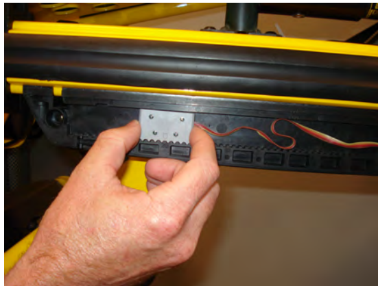
Figure 11 – Adjust left sensor height
