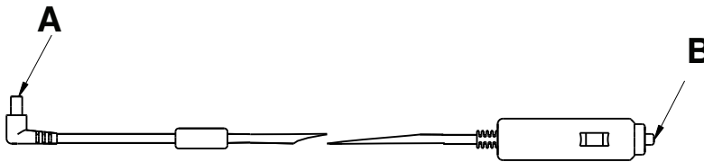
Figure 17 – 12 VDC automotive cable
