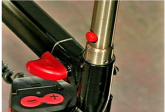
Figure 35a - Installed Push Bar
