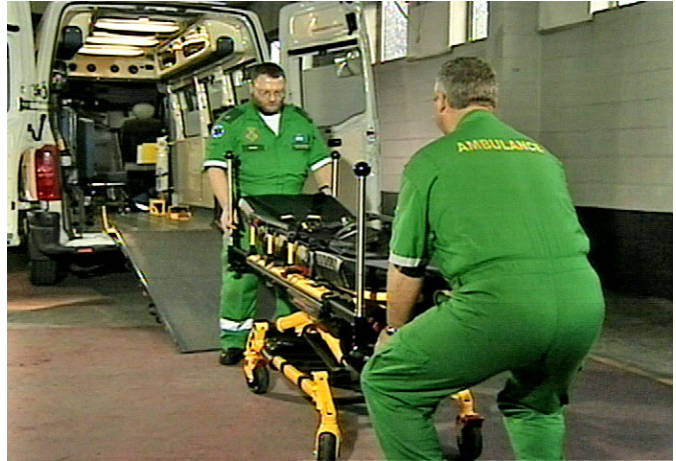
Figure 13 – Charger la civière
