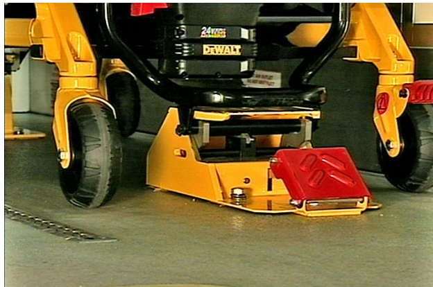
Figure 6 - Cot in Fastener - (Foot End)
