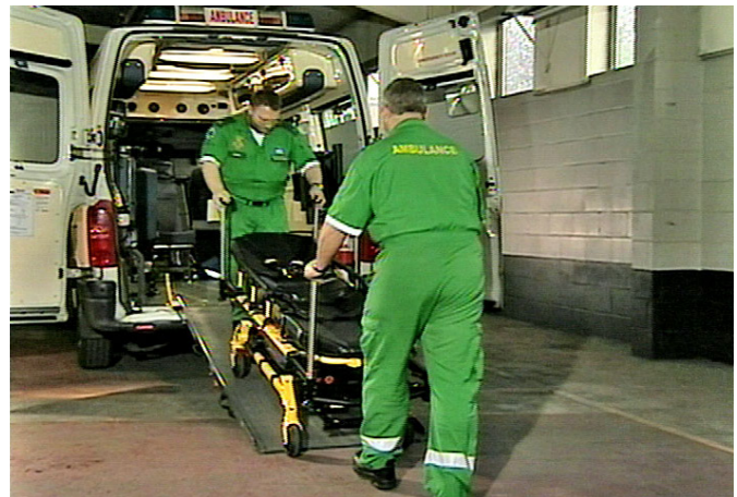
Figure 14 - Push Cot in Patient Compartment
