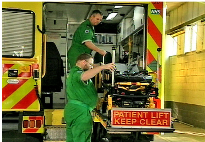
Figure 12 - Push Cot in Patient Compartment
