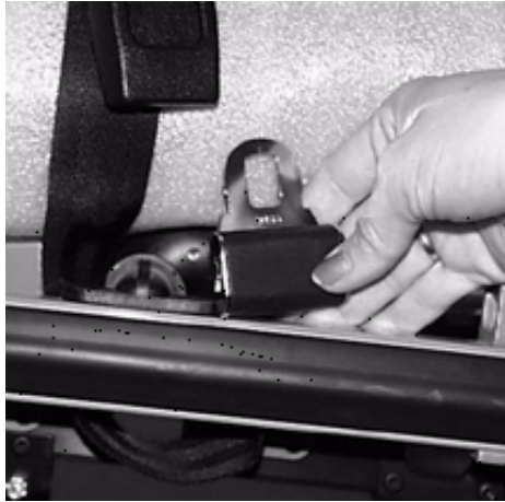
Figure 25 - Securing the Safety Restraints on a Cot
