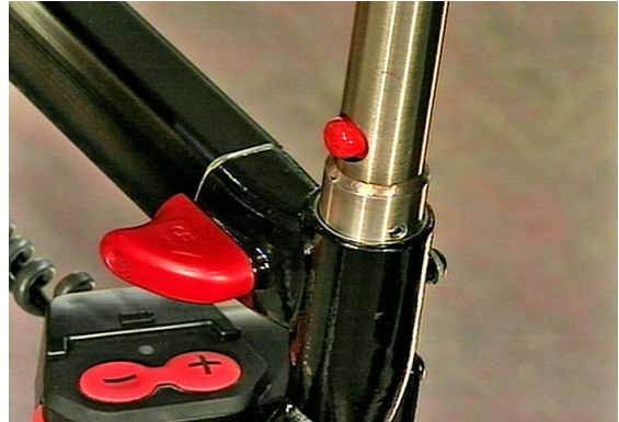
Figure 38 - Installed Push Bar
