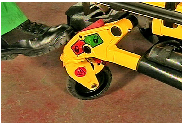
Figure 32 - Engage Caster Steer Lock
