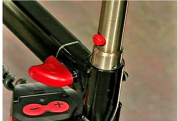
Figure 28.1: Installed Push Bar
