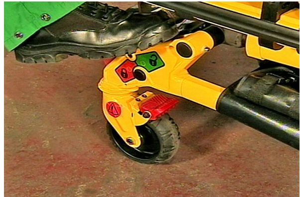
Figure 27.2: Disengage Caster Steer Lock
