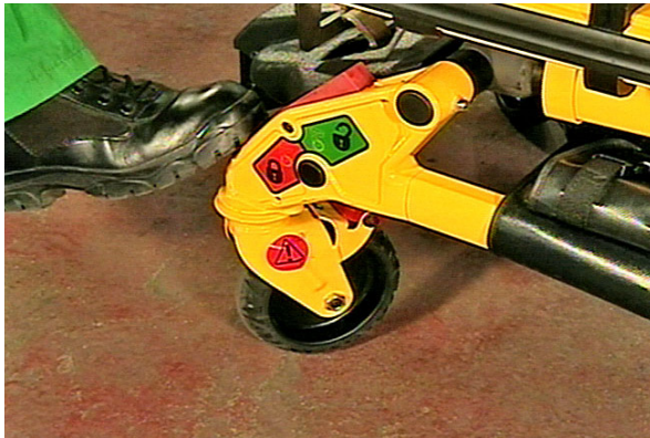
Figure 27.1: Engage Caster Steer Lock
