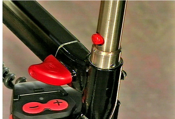
Figure 28.1: Installed Push Bar
