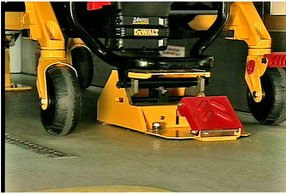
Figure 8 – Cot in both the head end and foot end of the cot fastener
