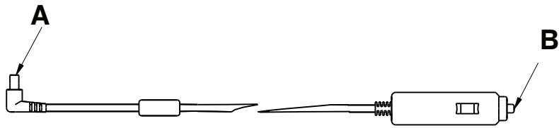
Figure 12 – 12 VDC automotive cable
