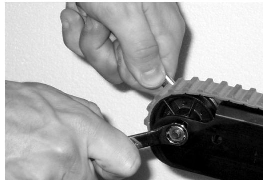
Figure 66 – Use wrenches to apply tension to the belt
