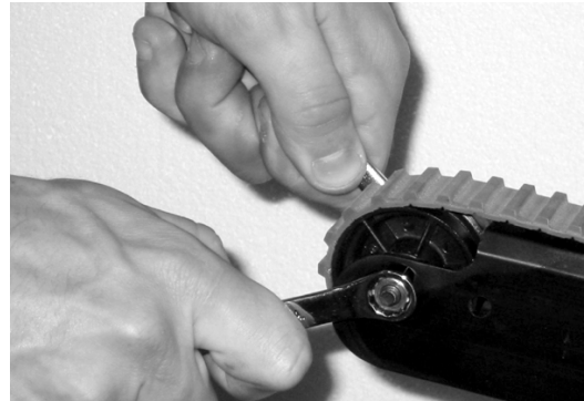
Figure 53 – Use wrenches to apply tension to the belts
