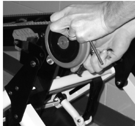
Figure 56 – Remove the wheel assembly
