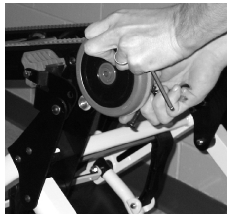
Figure 48 – Remove the wheel assembly
