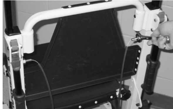
Figure 60 – Attach one side of the new cable
