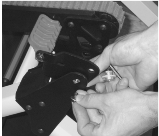
Figure 49 – Remove the track spacer pivots
