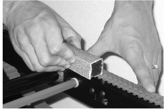
Figure 64 – Sand the wear surfaces
