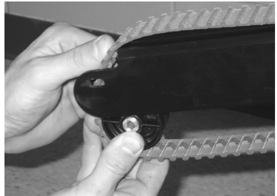
Figure 50 – Remove the rollers
