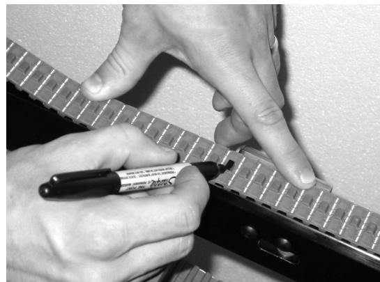
Figure 63 – Mark a belt tooth for reference
