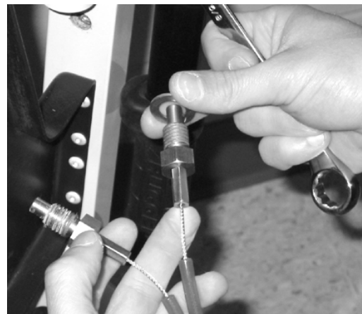
Figure 59 – Place the washer on the new cable
