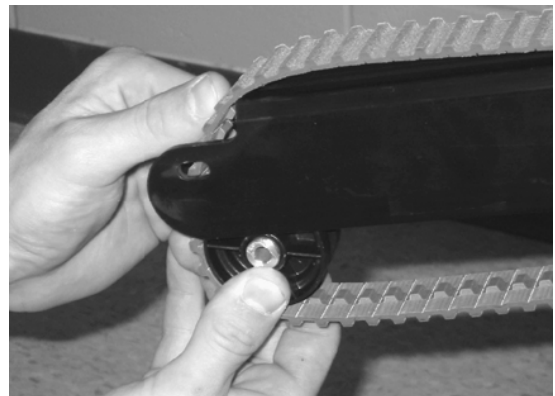
Figure 50 - Remove the rollers
