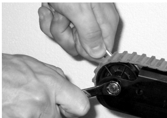
Figure 53 - Use wrenches to apply tension to the belts
