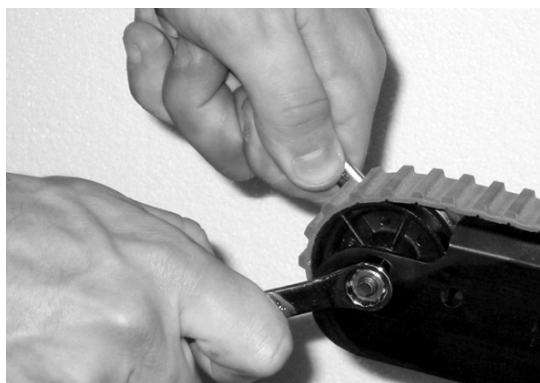
Figure 60 - Use wrenches to apply tension to the belt
