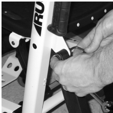
Figure 46 - Remove the screw, nut and washer
