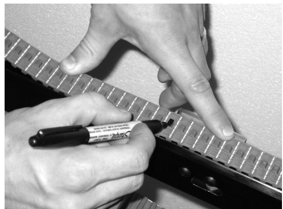
Figure 57 - Mark a belt tooth for reference
