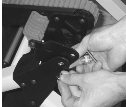
Figure 49 - Remove the track spacer pivots
