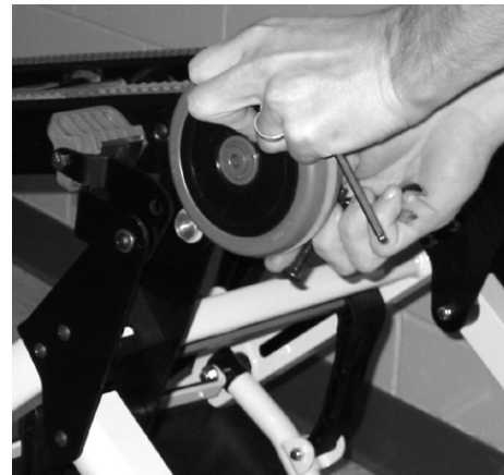
Figure 63 - Remove the wheel assembly
