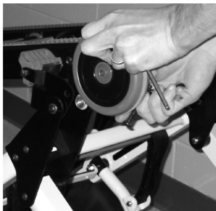
Figure 48 - Remove the wheel assembly
