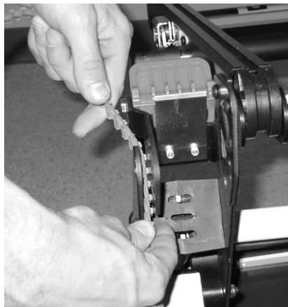
Figure 52 - Attach the new track belt
