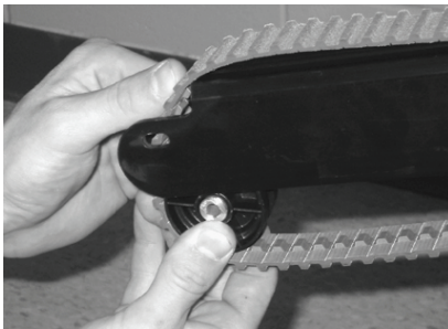
Figure 8 – Retirer les galets
