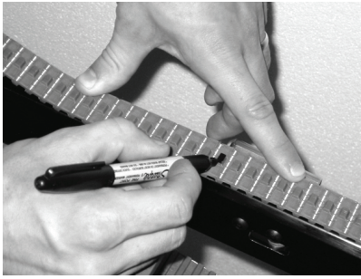
Figure 15 – Mark a belt tooth for reference
