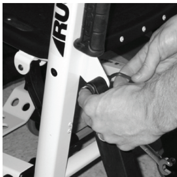
Figure 4 – Remove the screw, nut, and washer
