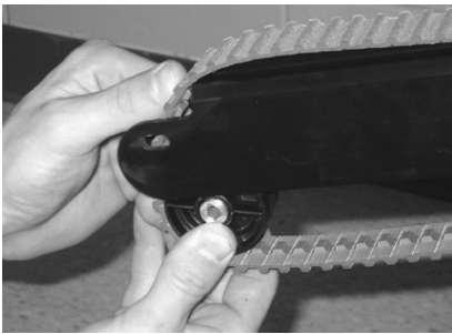
Figure 8 – Remove the rollers
