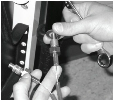
Figure 25 – Place the washer on the new cable
