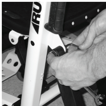
Figure 4 – Remove the screw, nut, and washer
