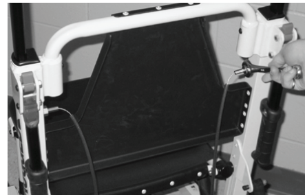
Figure 26 – Attach one side of the new cable
