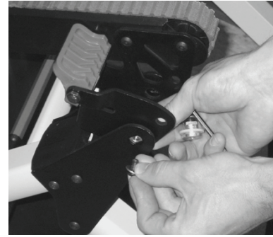
Figure 7 – Remove the track spacer pivots
