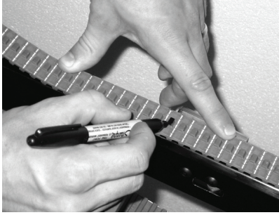
Figure 15 – Mark a belt tooth for reference
