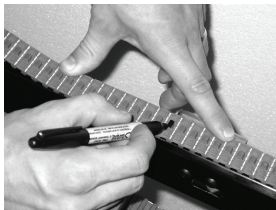
Figure 15 – Mark a belt tooth for reference
