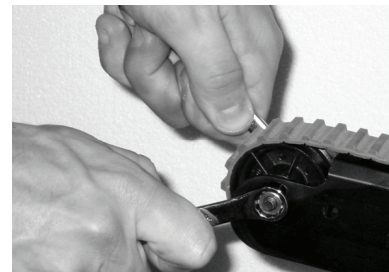
Figure 11 – Use wrenches to apply tension to the belts
