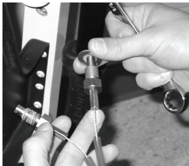
Figure 25 – Place the washer on the new cable
