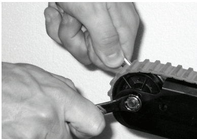
Figure 18 – Use wrenches to apply tension to the belt
