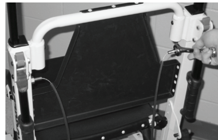
Figure 26 – Attach one side of the new cable
