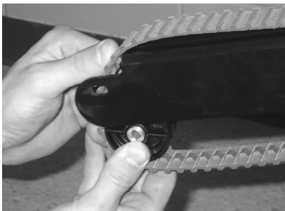
Figure 8 – Remove the rollers
