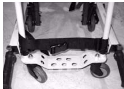
Figure 9-17 - Attaching the leg strap
