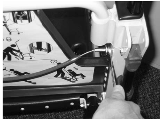
Figure 50 - Remove one side of the cable
