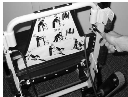
Figure 52 - Attach one side of the new cable
