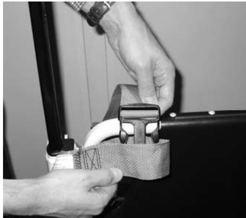
Figure 4 - Insert the end through the loop
