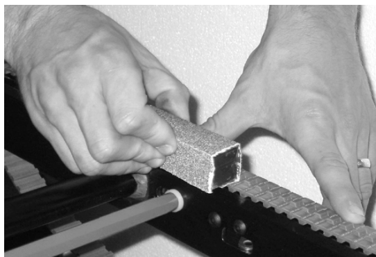
Figure 45 - Sand the wear surfaces
