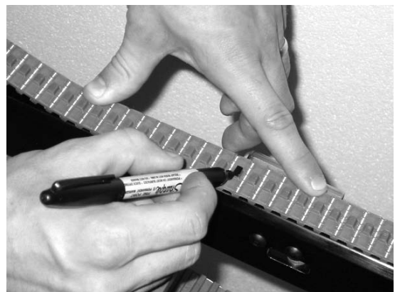
Figure 44 - Mark a belt tooth for reference
