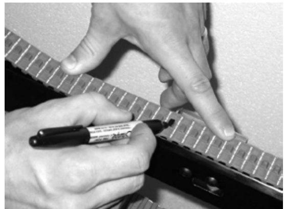
Figure 44: Mark a belt tooth for reference
