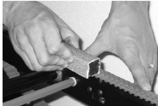
Figure 45: Sand the wear surfaces
