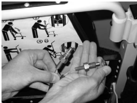
Figure 51: Place the washer on the new cable
