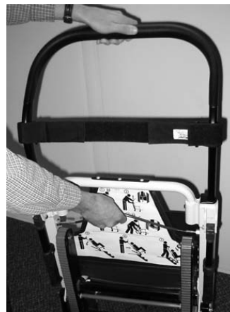
Figure 49 - Raise the extendable handle
