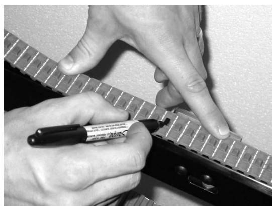
Figure 44 - Mark a belt tooth for reference
